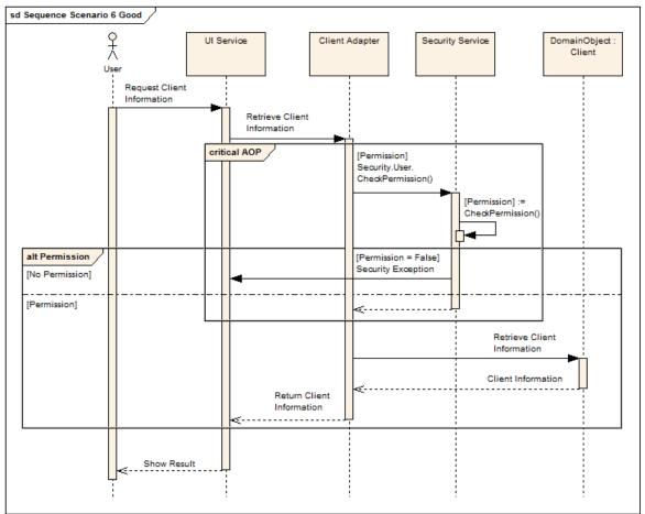
Figure 20: The authorisation sequence with the Client adapter and AOP
