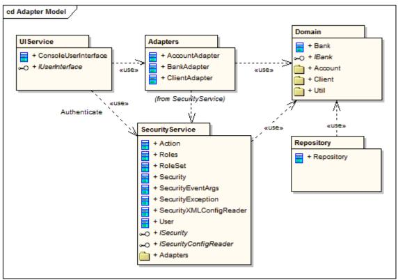
Figure 23: Class diagram of the adapter implementation
