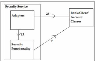
Figure 28: Coupling in the adapter implementation
