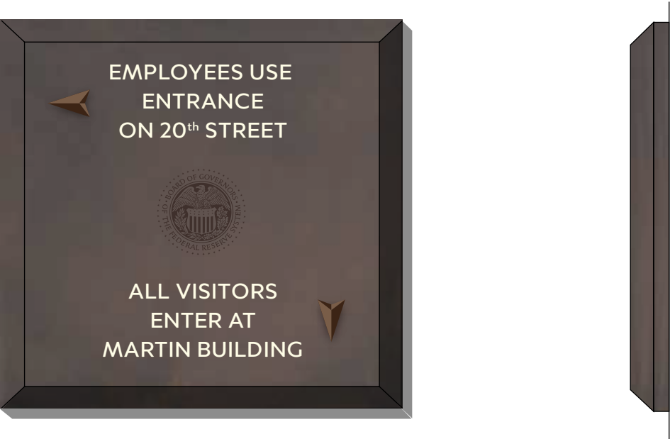
Figure 3-82: Detail Minimal Dark Bronze Plaque With White Applied Text And Etched FRB Seal. Plaque Attached Directly To Existing Facade
