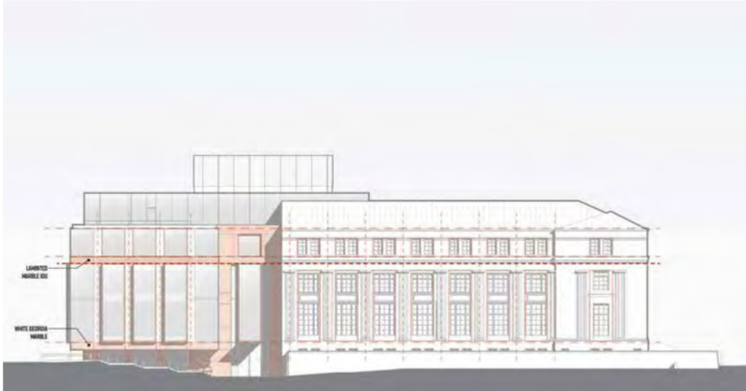
Figure 3-13: Tying new addition into FRB-East Building through the use of white Georgian marble
