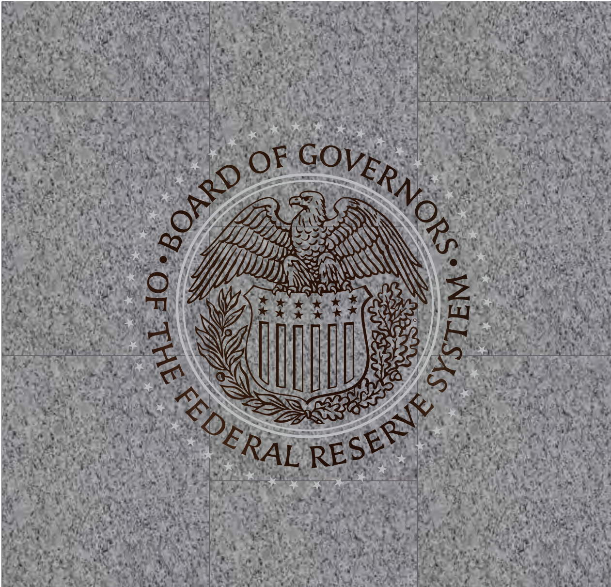
Figure 3-72: Detail Option 2 Seal Eagle And Lettering Fabricated From Dark Bronze Metal Inlaid Into Stone Pavers With Decorative Line And Star Borders Etched Into Stone Pavers
