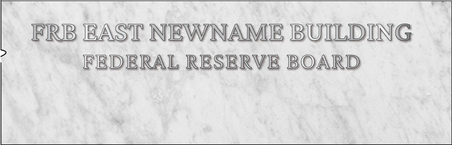
Figure 3-79: Detail Dimensional Letters Fabricated From Stainless Steel With Directional Bead Blast Finish And Pin Mounted
