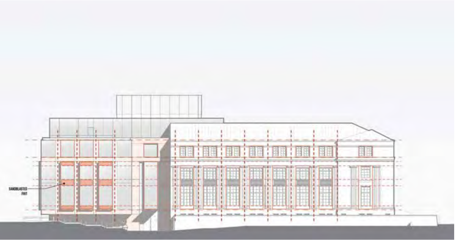
Figure 3-12: Reproducing FRB-East Building window spandrels through fritted glass
